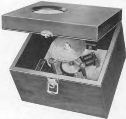
FIGURE 3. This synchronous motor is portable and connected to subsidiary amplifier circuits by a flexible cable. The disc makes use of transmitted light
