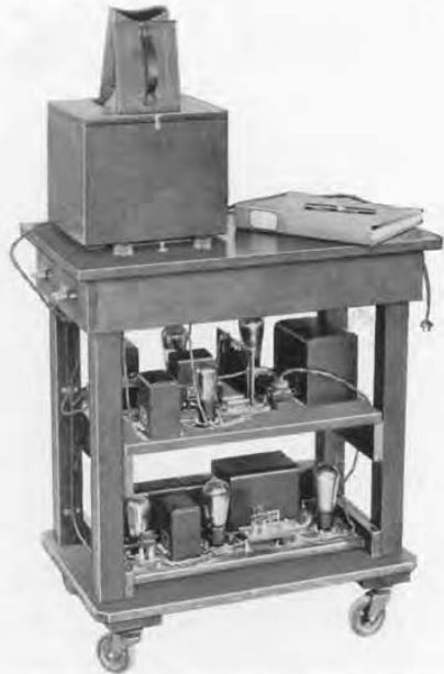
FIGURE 4. An experimental model of the stroboscopic frequency meter. Amplifier and power-supply circuits have been assembled with the synchronous motor on a cast-iron table
